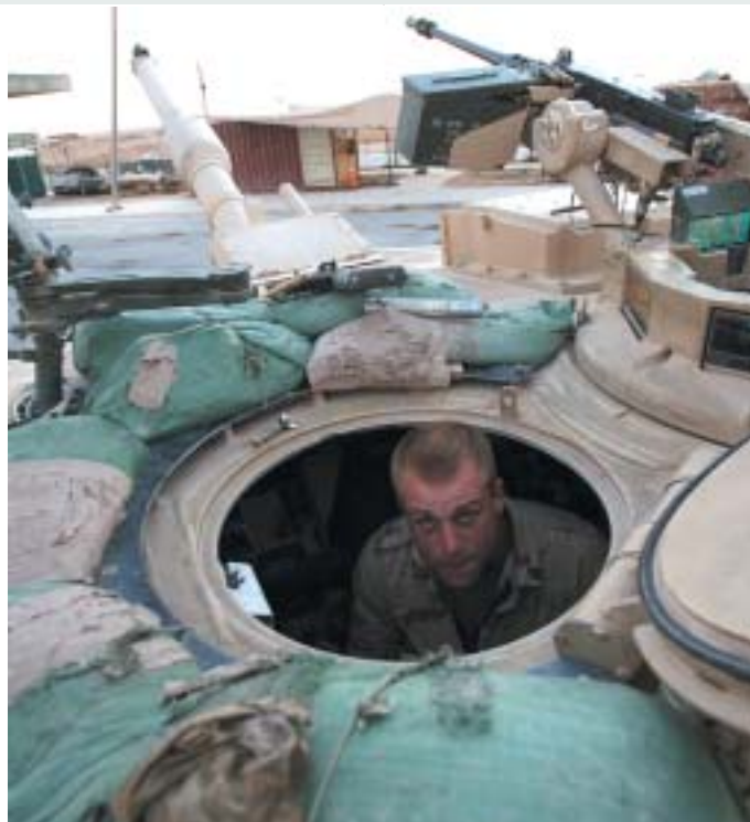
UPGRADING THE 'WORLD'S BEST' TANKS: In direct response to increasingly lethal attacks in Iraq, US Marines have resorted to raising M1A1 'Abrams' tank protection levels by adding layers of sandbags. The 2006 DCU has identified a raft of more sophisticated 'force protection' initiatives for the Australian Defence Force. USMC PHOTO
