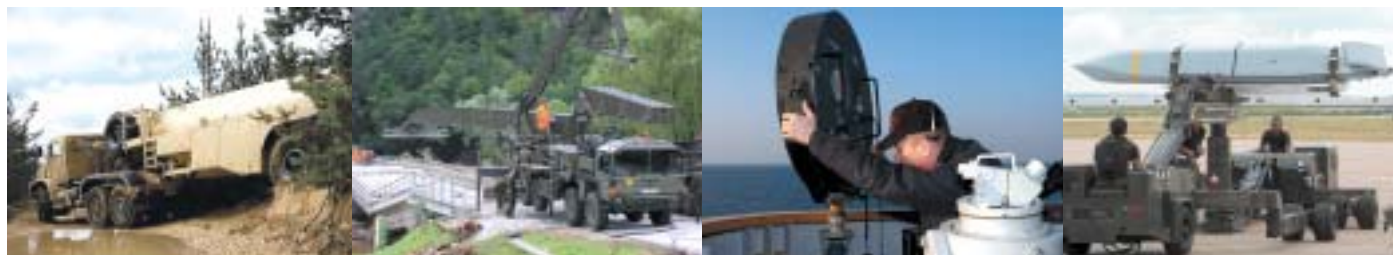
NEW CAPABILITY GRAB BAG IN FUTURE DCPs: Likely new initiatives to expand ADF capabilities coming in future budgets range from acquiring high mobility Aviation Refuelling Trucks like the 14,990 litre capacity MTVR-based tactical aircraft refueller adopted by the UK RAF (far left), mechanically deployed 'lines-of-communications' bridges (left centre), expanded Non-Lethal Weapons like this LRAD acoustic system (right centre), and enhanced weapons with potential to double existing strike ranges (ie: to in excess of 1,000km), as offered by the new JASSM-ER missile (far right).
